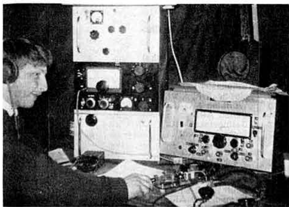
G3RTU operating G3HOX/P at Heaton Park, Manchester. Transmitter 10W to TT11 p.a. Receiver, double conversion, all home built. Aerial ground plane for 14 Mc/s. (Photo by G3CAG)
